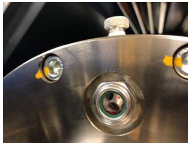
Sight glass for oil level in motor housing
